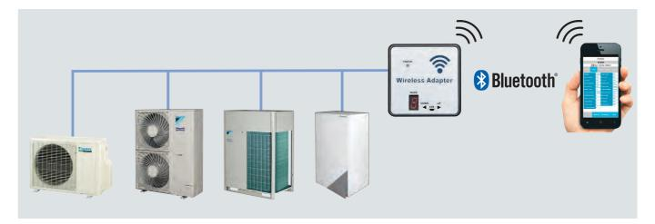
BTSC/i2S communicates with Split, SkyAir, VRV, Altherma indoor unit (Hydrobox) to service diagnosis, record operation data\*
