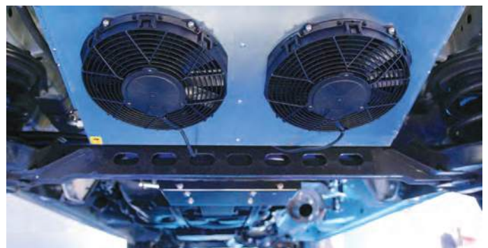
Installation of the SFZ 009e condenser in the back of the vehicle.
