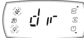
**Result:** The display shows "dir". The buttons that are on steady indicate that the corresponding actuator/function is active. The buttons that are flashing indicate that the actuator/function is not active.
