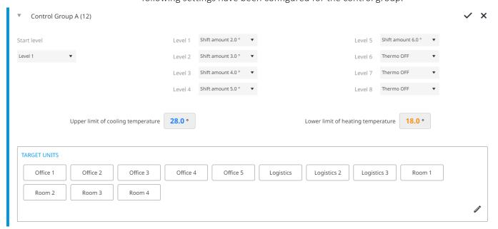
Daikin Cloud Plus reads out the Pi power consumption and imposes an increase in cutoff level as to not exceed the target demand value. Cutoff level 1 is triggered, and a temperature shift of 2°C is applied. The setpoint is changed to 20°C. When cutoff level 2 is triggered, a temperature shift of 3°C is applied and the setpoint is changed to 19°C.
