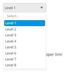
**6** Select a setpoint Shift amount (0~16°C, 1°C increments, or ThermoOFF) from the drop-down list for each cutoff level.
