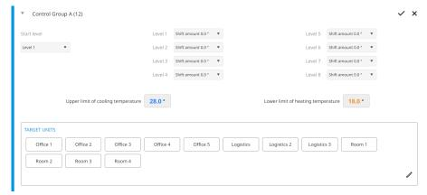
5 Select a Start level from the drop-down list. This is the cutoff level at which the setpoint control will begin (8 levels are available).
