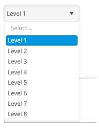
6 Select the capacity from the drop-down list for each cutoff level. This value (in %) determines how much capacity of the outdoor unit is able to utilise at each given cutoff level.
