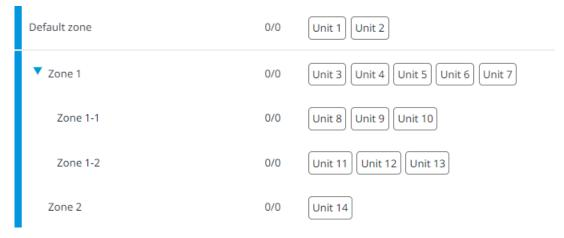
Since units can only belong to a single zone at a time, when an action is applied to zone 1, the action will only be applied to the units on that zone level (i.e. unit  $3^{7}$ ). The action is NOT applied to zone 1-1 (unit 8~10) or zone 1-2 (unit 11~12).
