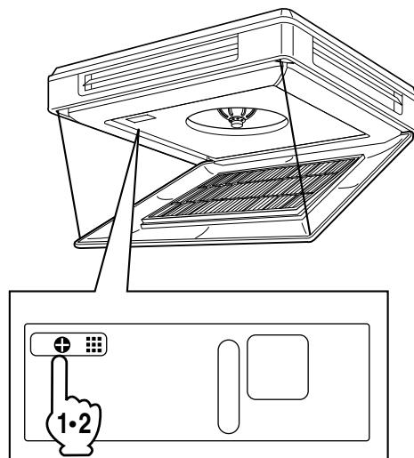
The local start button can be seen in the upper left-hand corner when the air intake grille is open.
