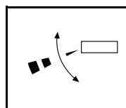
DISPLAY appears and the air flow direction continuously varies. (Automatic swing setting)
