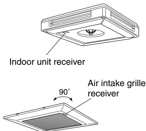
Turn the air intake grille 90° and attach to the indoor unit.
