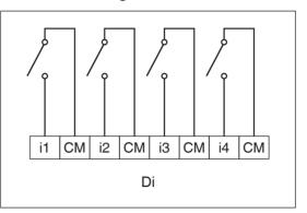
[i1] [i2] [i3] [i4] Pulse input, contact signal input [CM] Common
