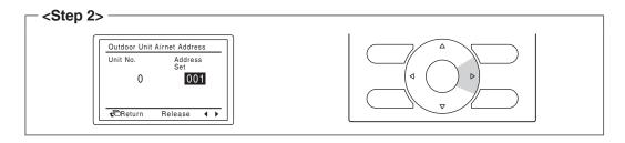
3. If an address is already [Set], press the Menu/OK button to release the current address setting. The mode indication changes from [Set] to [Release], and you are now ready to change the address.
