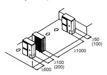
In case of installing multiple units (2 units or more) in lateral connection per row.
