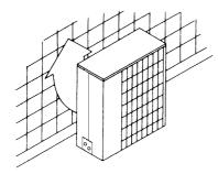
Set the outlet side at a right angle to the direction of the wind.
