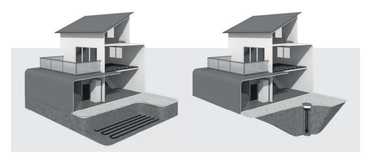
Geothermal energy is a free energy source for central heating and domestic hot water. This energy can be harnessed using geothermal collectors (left) or a geothermal probe (right).
