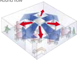
360° radial round flow enables uniform air flow distribution
