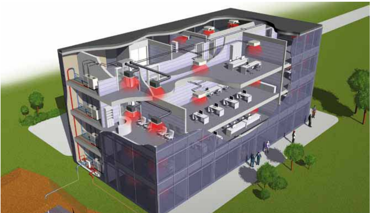
➡ Scheme of a water to air VRV® heat pump, using ground water (geothermal) energy as a renewable energy source.
